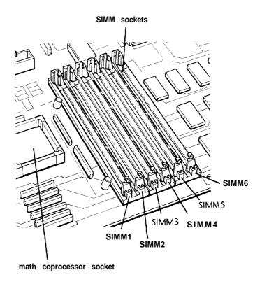
4. Remove the SIMMs in the sockets closest to the left side of the main system board first. Use your fingers or two small screwdrivers to pull away the tabs that secure the SIMM at each end. Be careful not to pull the tabs too far, or they may break.
